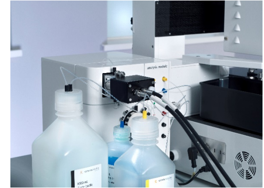
connection of a Tornado Raman Spectrometer
