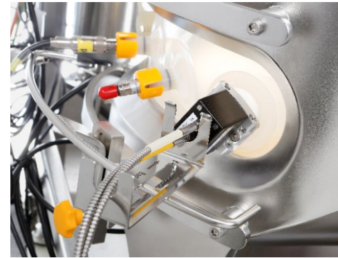
connection of a Tornado Raman Spectrometer
