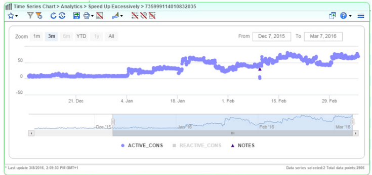
A broken meter showing an increased reading with constant consumption.
