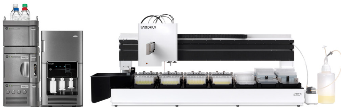
Scheme 1: A Schematic Illustration of BioAccord™ LC-MS System and Ambr® 15 High Throughput Bioreactor System.
