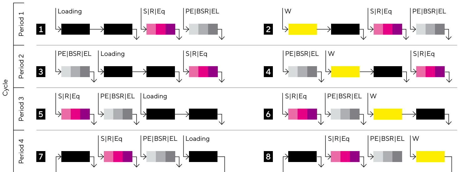
Figure 2: Purification in SMCC-Mode With Four Columns (L = Loading, W = Wash, PE = Pre-Elution, BSR = Baseline Return, EL = Elution, S = Sanitisation, R = Regeneration, EQ = Equilibration)
