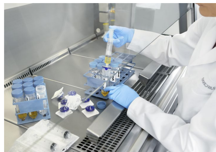
Figure 1: Initial clarification and subsequent sterile filtration of cell culture supernatants under aseptic conditions using a Minisart® High Flow syringe filter with a pore size of 0.22 µm.
