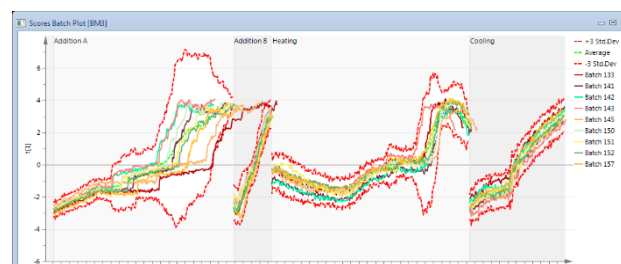
Figure 1: Multivariate batch control chart showing the model boundaries within each phase of the process and the evolution of the high performing batches.
