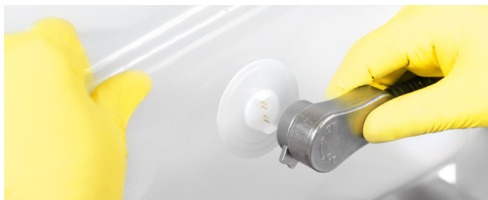
Figure 1: Viable Biomass Sensor (BioPAT® Viamass) Integrated in the Flexsafe® RM Bag – Connection to the Hardware Component.
