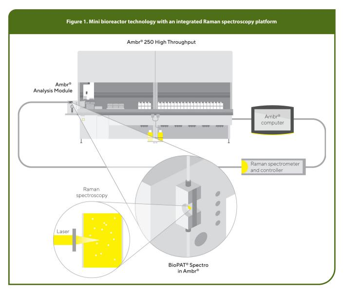
GlaxoSmithKline are working with integrated Raman spectroscopy from mini bioreactors through to manufacturing vessels to rapidly and more easily build models that can control their bioreactors. <sup>13</sup> Having this integrated real-time PAT technology from process development though to manufacturing scale will help to build Bioprocessing 4.0 upstream cell culture processes in many biopharmaceutical companies in future.
