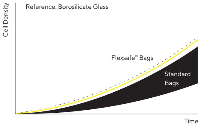
To ensure consistent cell growth performance, we optimized the resin and minimized the additive package in collaboration with our resin and film suppliers. The bags are proven to be free of cytotoxic leachables by independent labs. No bDtBPP identified in WFI extract of Flexsafe® bags.
