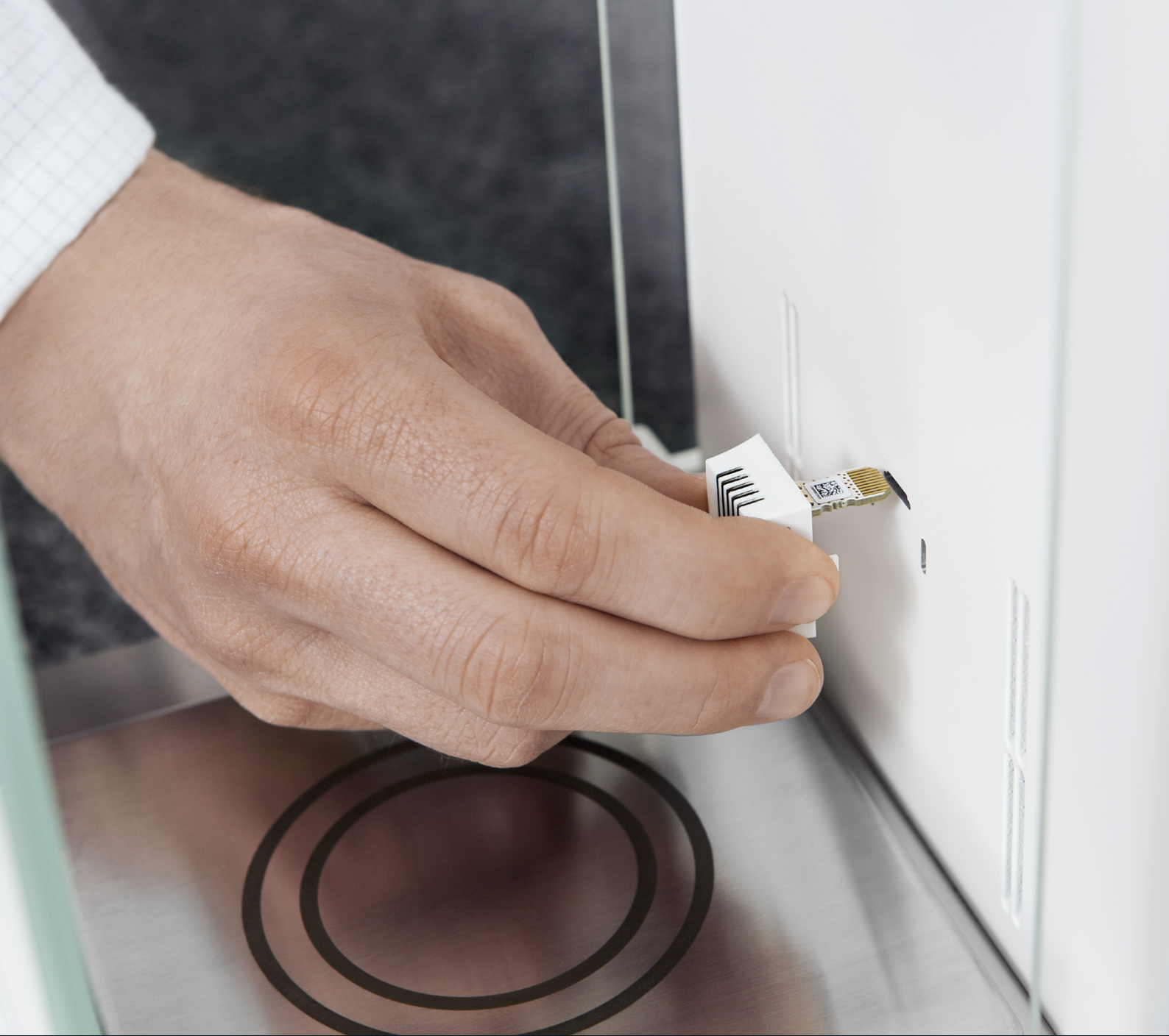
Climate module connected within the draft shield
