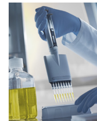
Figure 4: Bad pipetting technique, in particular in combination with mechanical pipettes with stiff plungers, increases the risk for cross-contamination. Sartorius Tacta pipettes have soft plungers, preventing retraction of contaminating droplets into the pipette. In comparison to the two pipettes from other manufacturers, cross-contamination was not observed with the 100-1000 µl Tacta pipette.
