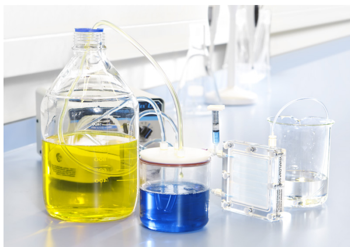
Fig. 2: Diafiltration system set up for buffer exchange. Culture medium concentrate can be seen in the center of the image. 1 L 25 mM Sodium Acetate (exchange buffer) can be seen connected to the system on the left of the image.
