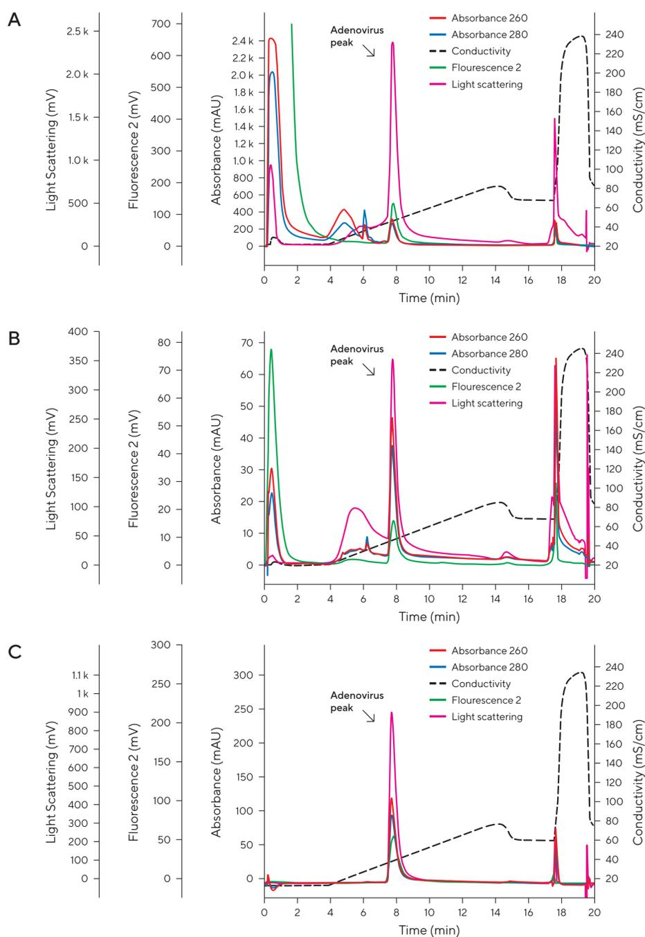
Note. Column: CIMac™ Adeno, Buffers: MPA: 20 mM BTP, 150 mM NaCl, 2 mM MgCl<sub>2</sub>, 1% sorbitol, 0.5% poloxamer, pH 8.5, MPB: 20 mM BTP, 1 M NaCl, 2 mM MgCl<sub>2</sub>, 1% sorbitol, 0.5% poloxamer, pH 8.5. Detection: UV absorbance (260, 280) PicoGreen fluorescence<sup>1</sup> (Pg-FLD) and MALS.
