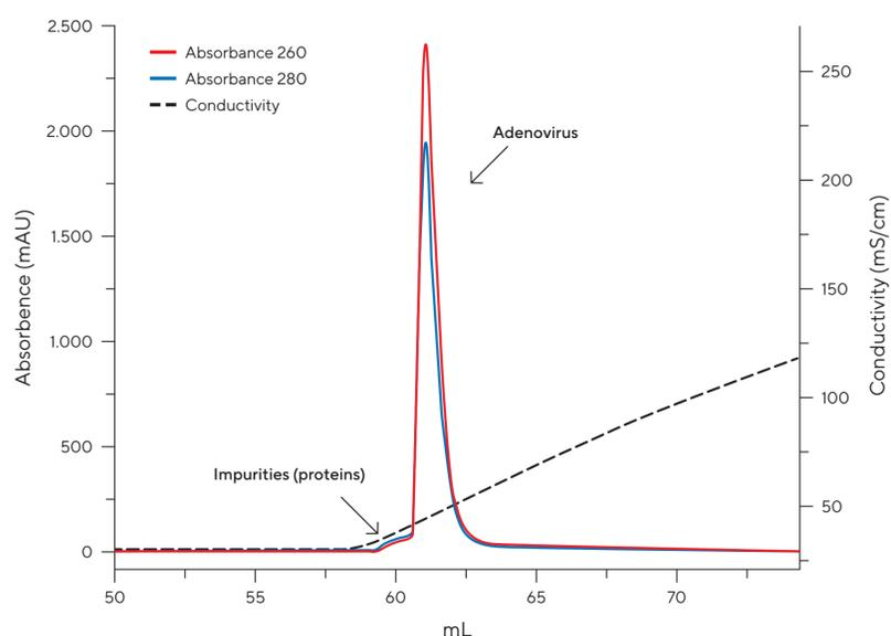
Note. Buffers: MPA: 50 mM Tris, 300 mM NaCl, 5% saccharose, 0.1% poloxamer 188, pH 8.5, MPB: 50 mM Tris, 2 M NaCl, 5% saccharose, 0.1% poloxamer 188, pH 8.5 | Sample: Adenovirus 5, TFF clarified retentate | Detection: absorbance (260, 280)
