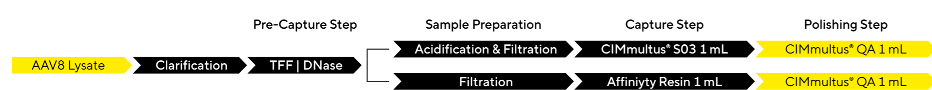
Figure 1: Schematic Diagram of the Purification Process
