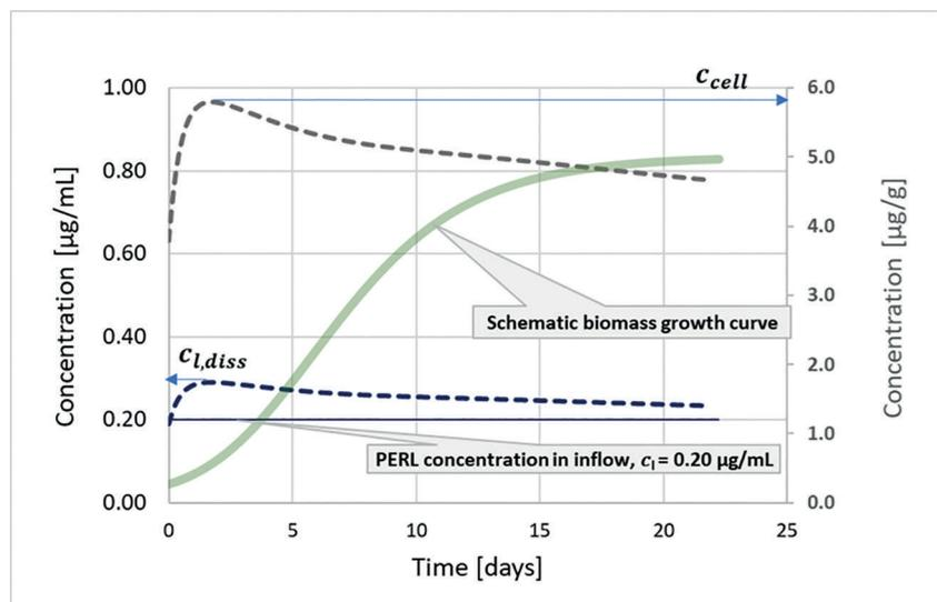
Figure 4: Modeling results of 2,4-DtBP exposure in a CGT perfusion bioreactor to the liquid phase (blue dashed curve) and the cellular phase (grey dashed curve). The green sigmoid curve represents a hypothetical cell growth used in this model. The flow is much higher than release rates of PERLs indicating a strong wash out effect; an accumulation of PERLs in the liquid and/or cellular phase does not occur.
