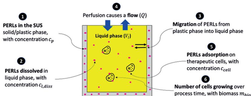
Figure 3: Scheme of a model perfusion bioreactor with 6 relevant processes for digital twin development to estimate PERL concentration.
