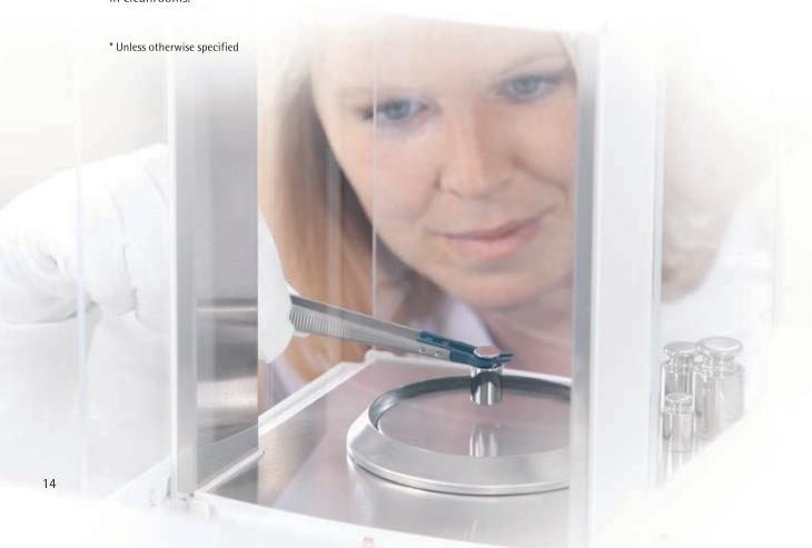
Sartorius Proof Line knob weights of OIML classes F1 and F2 with nominal values of 1 g and higher are made of stainless steel that has a density of 7,950 kg/m³. The tolerances of these knob weights comply with OIML R111-1 and they are supplied in high-quality plastic screw-top boxes. Knob weights from 10 g and up feature an adjustment chamber.
