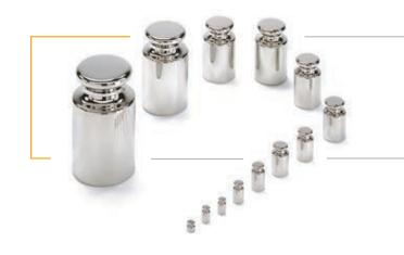
Proof Line OIML class F1 leaf weights ranging from 1 mg to 5 mg are made out of aluminum that has a density of 2,650 kg/m³; those with nominal values from 10 mg to 500 mg are manufactured from nickel silver that has a density of 8,600 kg/m³. Their tolerances comply with OIML R111-1.
