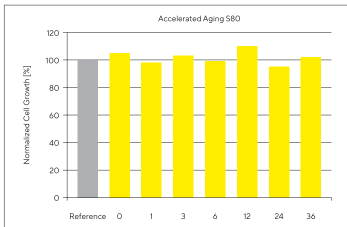
Figure 5: Cell growth testing of Flexsafe® against glass bottle reference during the three-year shelf life.
