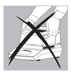
Never lift and carry the analyzer by its heating module.
