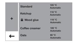
> The unlocked method is then displayed in the method menu without an ♠ symbol. It is available for selection and can be used for moisture analysis.
