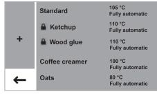
$\triangleright$  The locked method is then displayed in the method menu with an  $\triangle$  symbol. It is not available for selection and cannot be used for moisture analysis.
