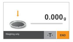
➤ The weighing screen appears.You can now use the moisture analyzer as a simple lab balance.
