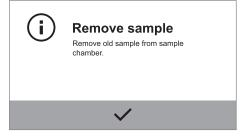
▶ When you have exited the measurement by selecting **OK**, you can remove the sample from the moisture analyzer.
