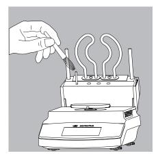
4) Clean the heating element and temperature sensor with a weak solvent such as ethanol.
