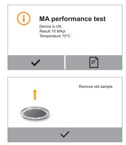
▷ If the test is successful, the message "Device is OK" first appears. Then the analyzer indicates that the sample can be removed.
