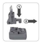
Push (1) and slide (2) the mains adapter required for your power supply into the opening of the AC adapter module. When doing this, the mains adapter needs to lock into position.
