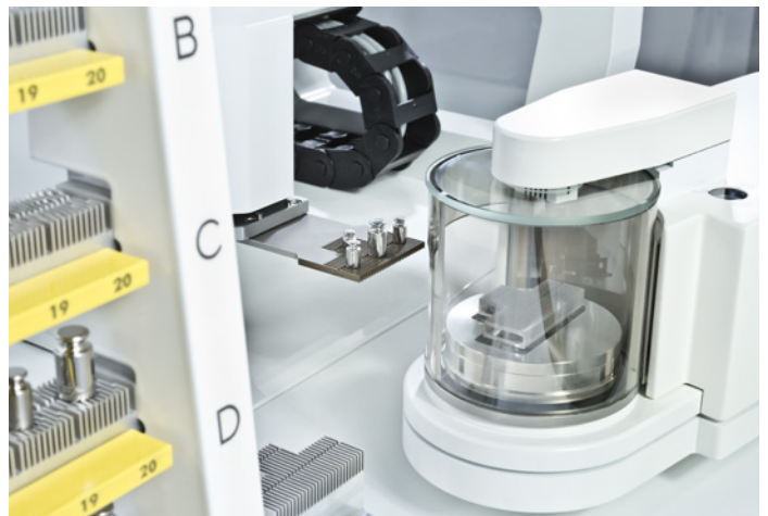
Picture 5: Weighing Cells are equipped with automatic doors
