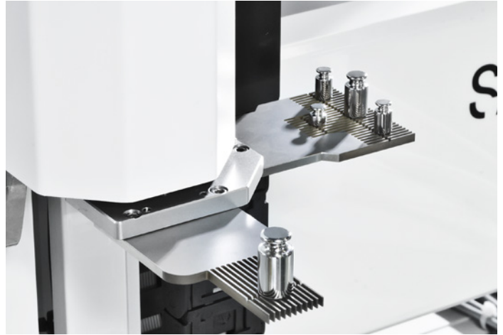
Picture 4: Dual arm system with multi-weight-and single weight handlers
