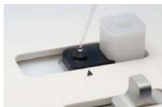
Figure 5-22: Adding 4 \mu\text{L} of Sample Diluent into Drop Holder
