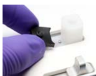
Figure 3-3: Placing a Drop Holder on the BLItz System (press gently to ensure a snug fit)
