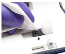
Figure 5-16: Wiping the Drop Holder with a Kimwipe
