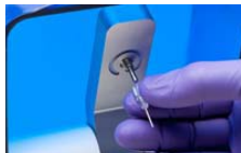
Figure 5-36: Mounting a Biosensor
