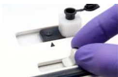
Figure 5-37: Moving Slider to Bring Drop Holder or Tube to the Read Position
