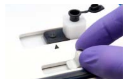
Figure 5-24: Moving Drop Holder to the Read Position
