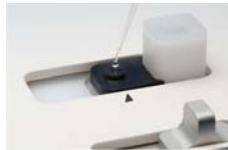
Figure 5-35: Adding 4 \mu\text{L} of Sample Diluent into Drop Holder
