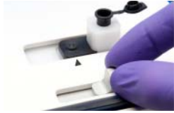
Figure 5-12: Moving Drop Holder to Read Position
