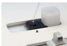
Figure 5-10: Adding 4 µL of Sample into Drop Holder
