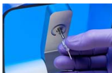
Figure 5-11: Mounting a Biosensor
