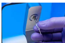
Figure 5-23: Mounting a Biosensor
