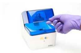
Figure 5-38: Closing the BLItz System Cover
