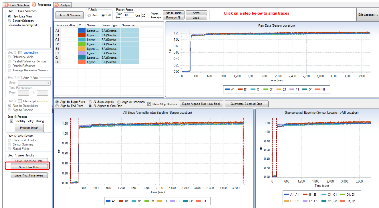
FIGURE 3.14. PROCESSING TAB OF OCTET DATA ANALYSIS SOFTWARE SHOWS AN EXAMPLE DATA SET FOR DRIFT TESTING.
