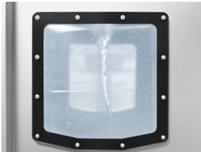
Fig. 8: Vortex at 475 rpm in a 200 L Flexsafe® Bag for Pro Mixer
